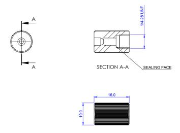
NOTE:- CONNECTION TUBE MUST NOT EXTEND BEYOND SEALING FACE
